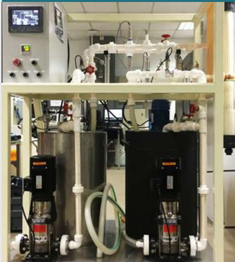
Bench scale oil water treatment system
