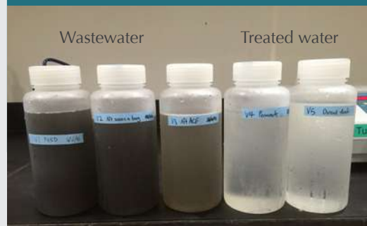
From car wash wastewater to high quality treated water
